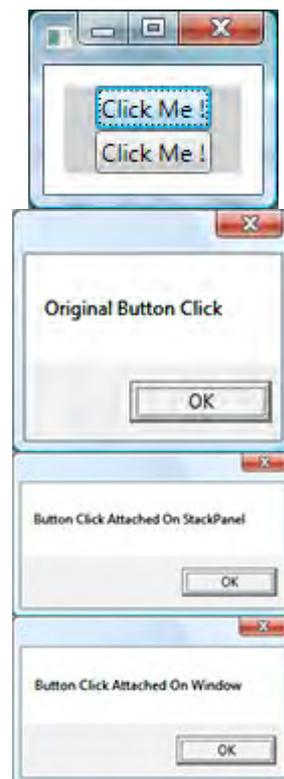
The sample handles the bubbling Click event raised by one of its Buttons on the StackPanel and on the root Window level. Because neither StackPanel nor Window define their own Click events, the event attribute names **Click** must be prefixed with the class name **Button.Click**.
