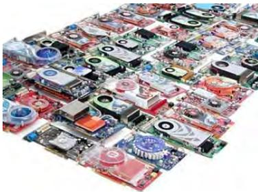
In most cases a graphics card is an expansion board plugged into a slot on the motherboard.
